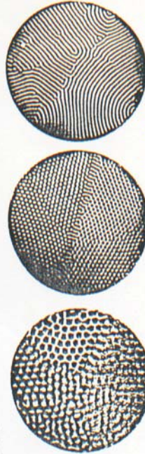
All shook up. A layer of particles shifts from one surface pattern to another as the vibration amplitude changes.
