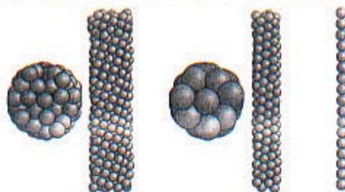
2 Simulations of a lead nanowire show that it can form a helical structure. The complete wire is shown on the left, the wire with the outer shell removed is shown in the middle, and the inner strand is shown on the right. The cylindrical shells are related by a kind of "curved surface epitaxy" between 2-D lattices that are otherwise incompatible.
